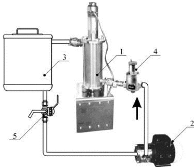
Experimental installation with the cavitation reactor of the company *Oil Tech Production OY*:
